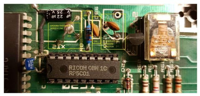
Last part is VCC supply and backup logic for the RTC chip, plus the resistor attached to /ALARM and ADJ. The R50 is replaced by a wired and an additional polarized capacitor is need CA1 (22uF 25V) and positive side is connected to the C62 (0.1uF marked as 104K) and the minus side (marked as -) is connected to ground. (IMPORTANT! will burn if connected wrong)
