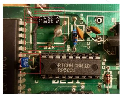
Use the scalped to remove some protected green shield from the ground line. (be carful just the shield not the copper)
